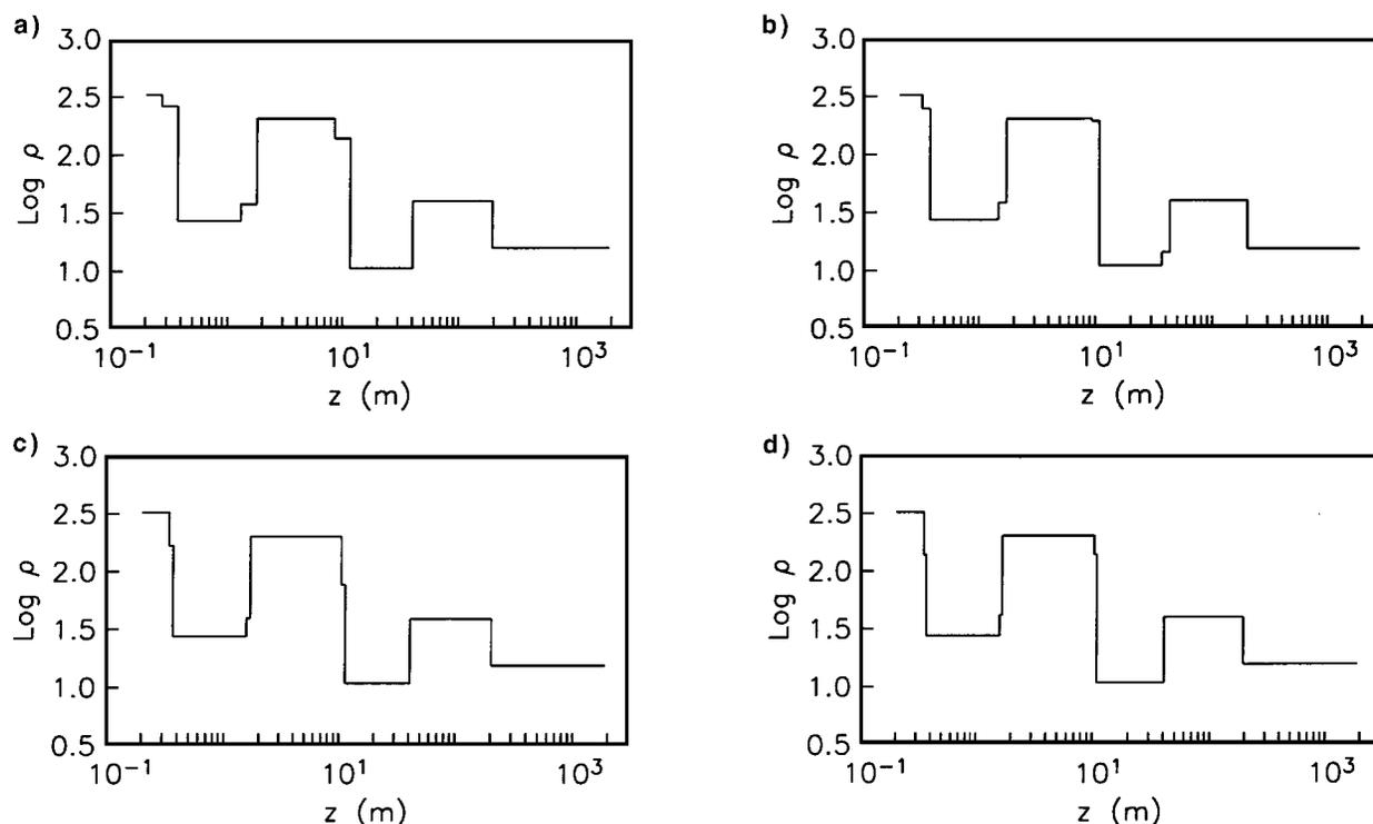
FIG. 2. Final models for four different discretizations of the depth axis. The models were obtained in six iterations using as data the sounding curve shown in Figure 1d. In all cases, the discretization begins at a depth of 0.2 m and ends at 1700 m. The intermediate depths follow geometric series defined by  $m$ , the number of unknowns. The models correspond to (a)  $m = 30$ , (b)  $m = 60$ , (c)  $m = 120$ , and (d)  $m = 180$ . The model shown in Figure 1 was obtained using  $m = 60$ .
