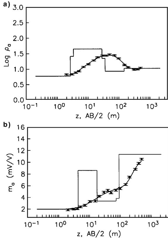
FIG. 5. Interpretation of a combined resistivity and IP sounding. This case differs from the one shown in Figure 4 in that the present resistivity curve has more character. (a) Resistivity data compared with the response of the final resistivity model. (b) IP data compared with the response of the IP model. In both cases, the models are plotted using the same scales as their corresponding data sets. The resistivity model was obtained in three iterations, and the IP model was obtained in one.
